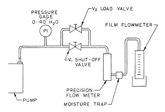
Figure 7 LFS-113 Sampler
